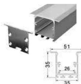
Recessed Aluminum Profile width 51*35 mm opening 35mm
