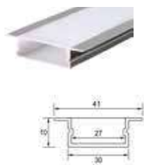
Recessed Aluminum Profile width 41*10 mm opening 30mm
