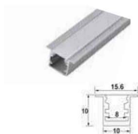
Recessed Aluminum Profile width 15*10 mm opening 10mm
